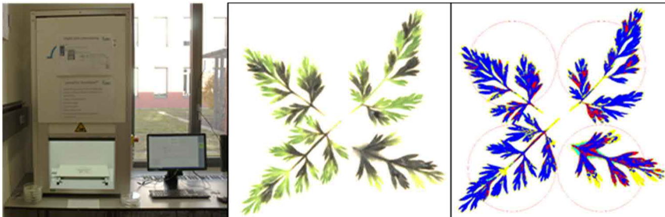
Lemnatec system (l.) digital picture with disease symptoms (m.) and color classification (r.) by the Lemnatec software
